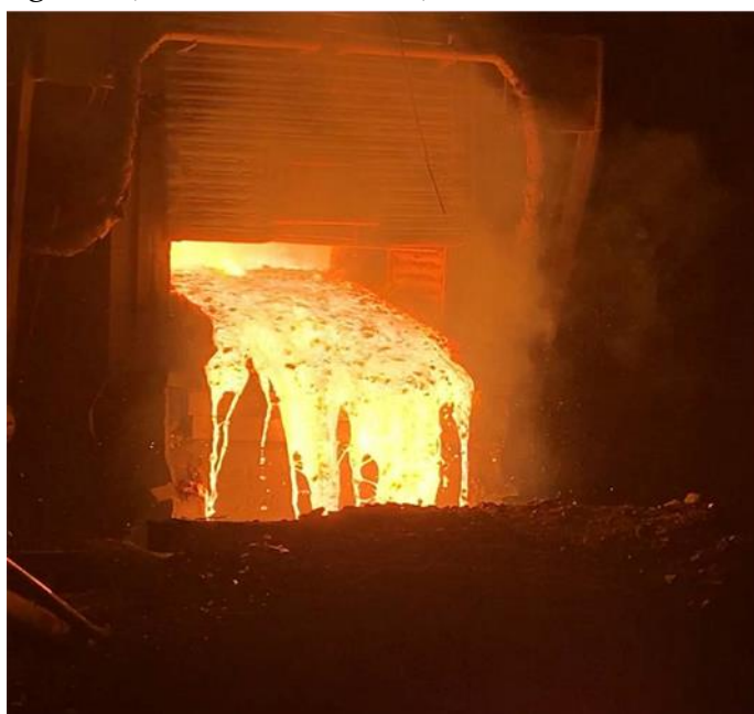
Figure 1. The Process Of Extracting Liquid Metal From A 30 – Ton Electric Arc Furnace
