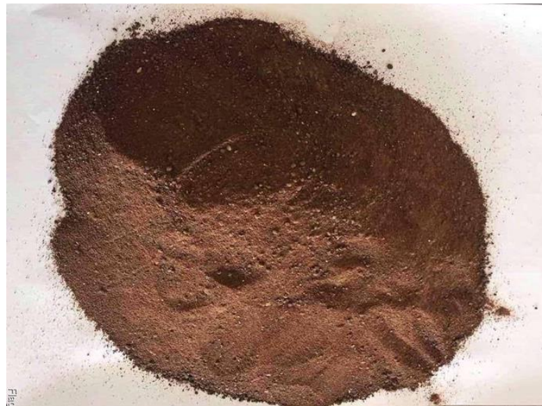
Figure 3. A mixture obtained by grinding refractory magnesite brick and slag into powder
