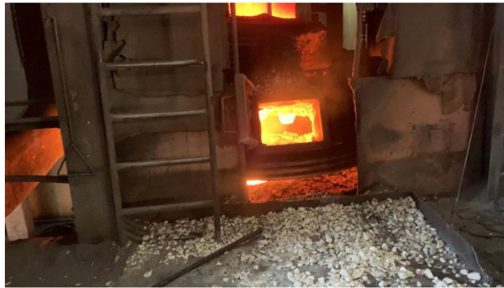
Figure 2. The process of restoring lining from the window of an electric arc furnace
